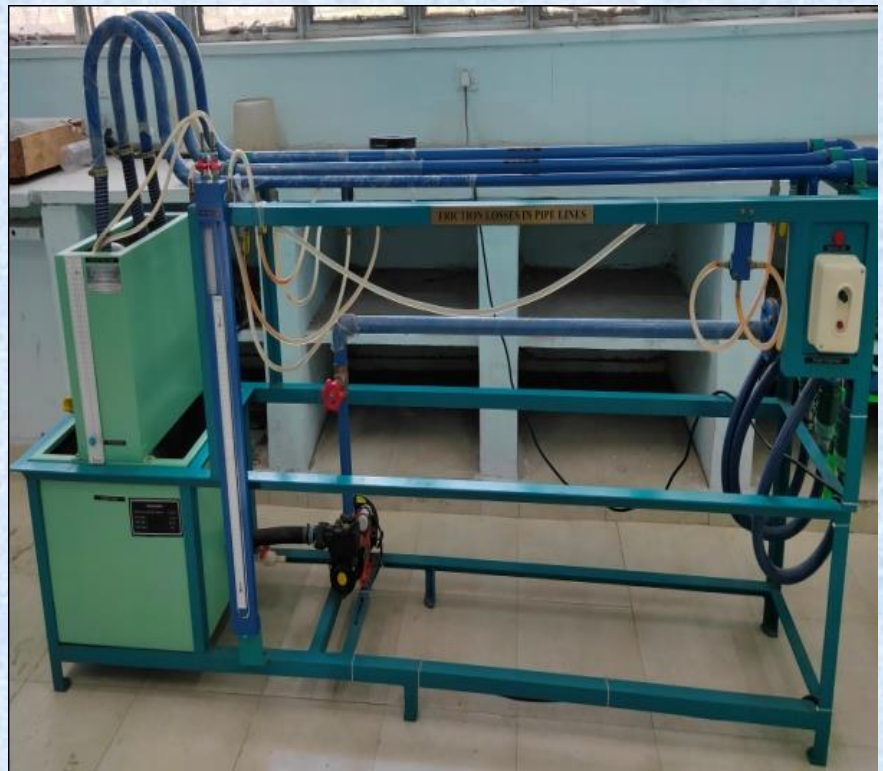
Friction Losses In Pipes Setup
